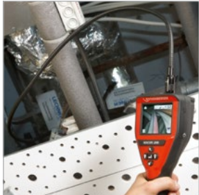
Camera head with high-performance LEDs
